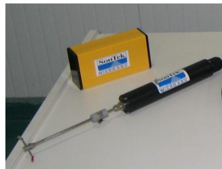
Figura 3.6. Sonda y receptor ADV
