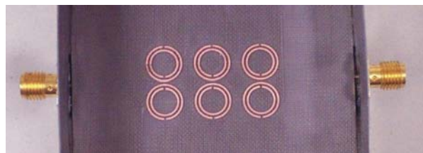
Fig. 7. Prototype of a metamaterial-based planar filter in coplanar waveguide technology using 3 unit cell SRR structure.
