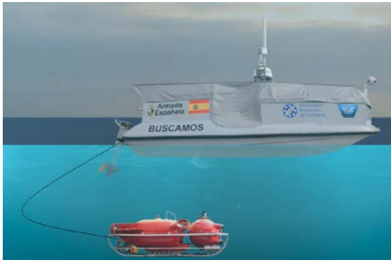
Fig. 1 BUSCAMOS-Oil system. Composed by an ASV and an UUV.
