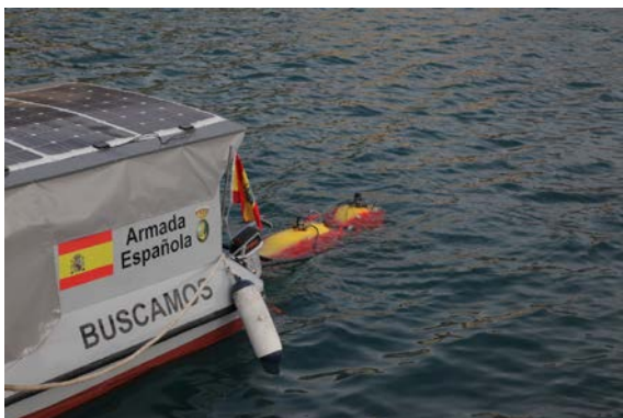
Fig 22. Launching the UUV.
