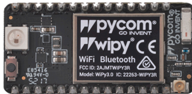
Figure 2. WiPy 3.0 development board based on ESP32 chip.
