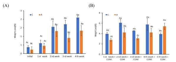
Figure 1. Weight loss of lemons stored in active (A) and control packages (C) for 5 weeks at 8 °C (88% RH) (A) and after supplementary commercialization periods (5 days at room temperature) (B). Different capital letters denote significant differences between packaging treatments for the same storage time. Different lowercase letters denote significant differences between storage times for the same packaging treatment.
