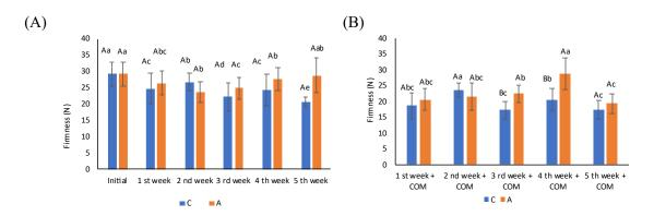
Figure 3. Firmness of lemons stored in active (A) and control (C) packages for 5 weeks at 8 °C (88 % RH) (Figure 3A) and supplementary commercialization periods (5 days at room temperature) (Figure 3B). Different capital letters denote significant differences between packaging treatments for the same storage time. Different lowercase letters denote significant differences between storage times for the same packaging treatment.
