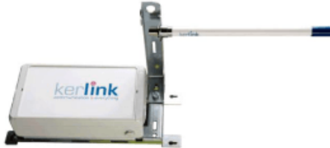
Figure 1.6 Kerlink Wirnet LoRa IoT Station
