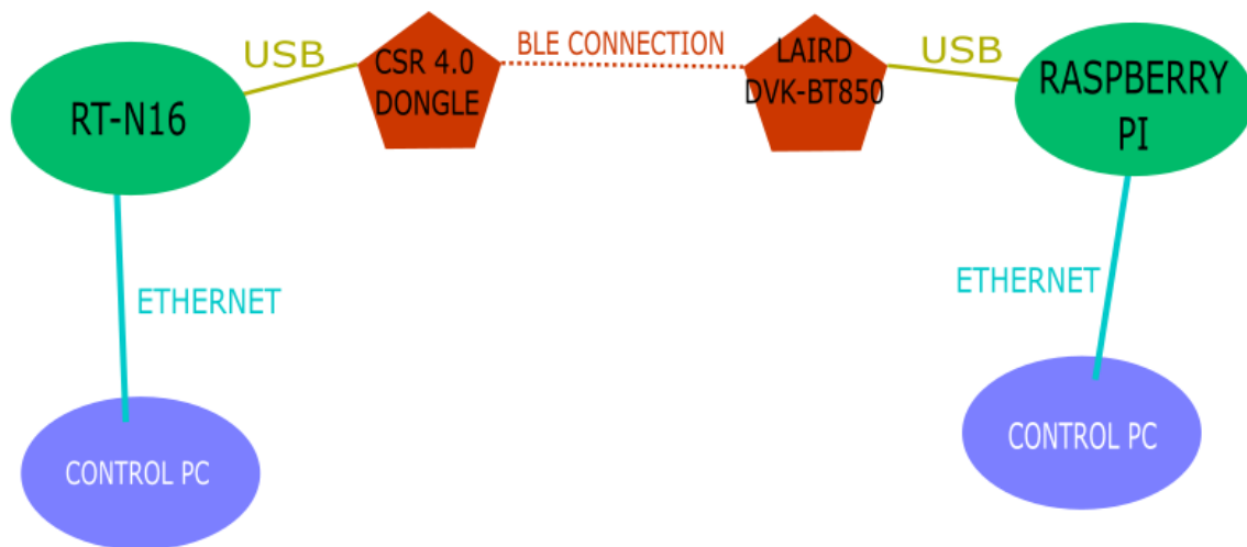
Figure 3.9 Topology to implement a BLE connection (II)
