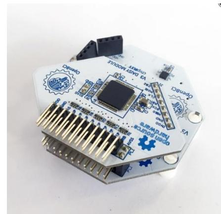
Figura 22. Dispositivo Cyton + Daisy Biosensing Board
