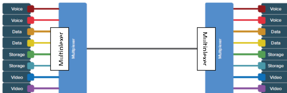
Fig. 11. Multiplexing combines multiple channels on a single fiber
