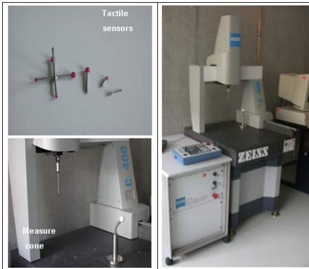
Figure 4.6 Sensors of coordinate measuring machine
