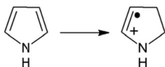
Figure 7: Initiation of the polymerization in pyrrole monomers.
