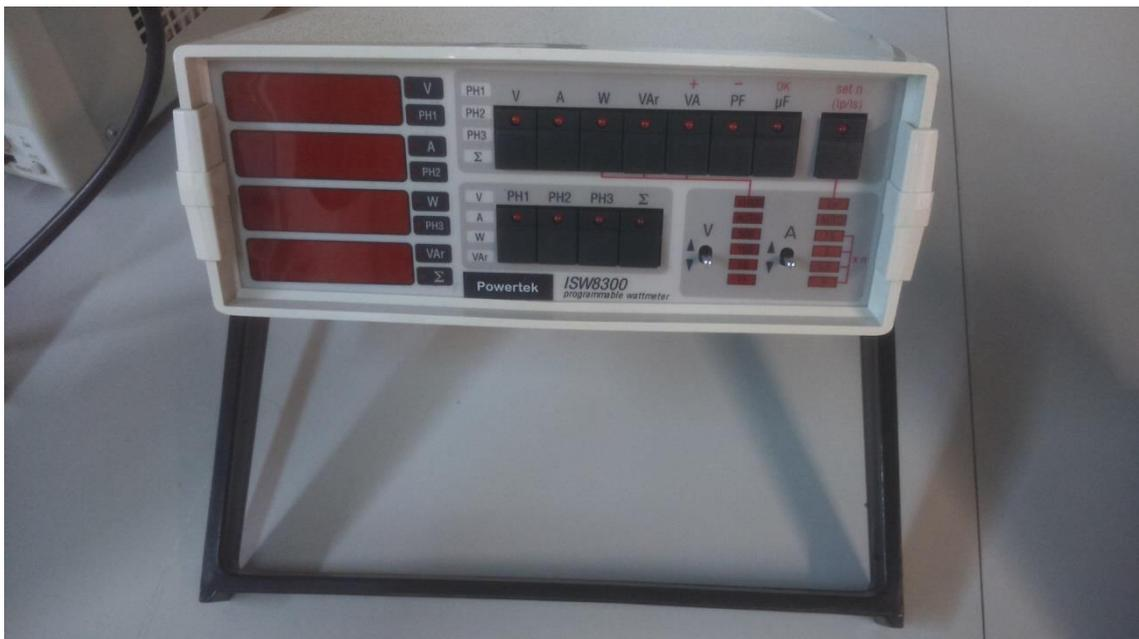
Figura 11: Wattímetro digital. Displays. Y control.
