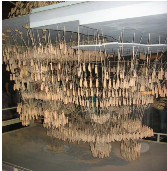
Figure 40: Poly-funicular miniature design by Gaudí – Sagrada Família Museum – Barcelona
