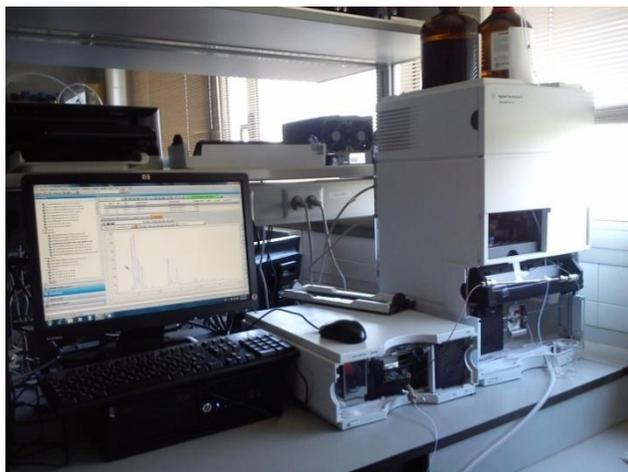
**Figura 7.** HPLC Agilent 1260 Infinity
