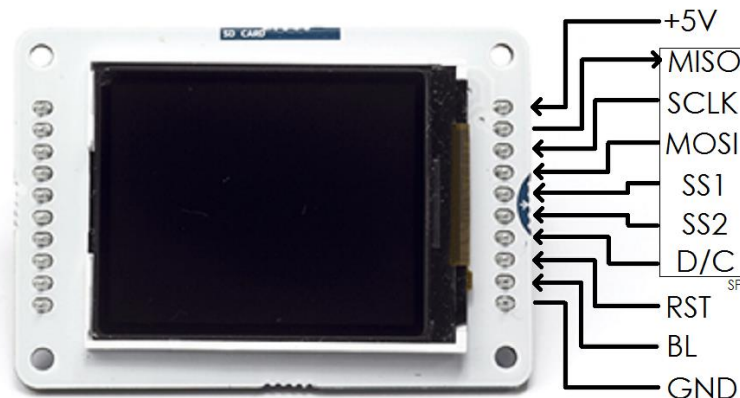
Figure 46. Arduino TFT LCD pinout [47].
