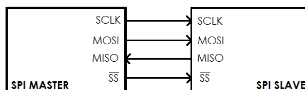
Figure 45. Typical single SPI bus master and slave 2 .
