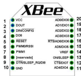
Figure 53. XBee Series 1 pinout [51].
