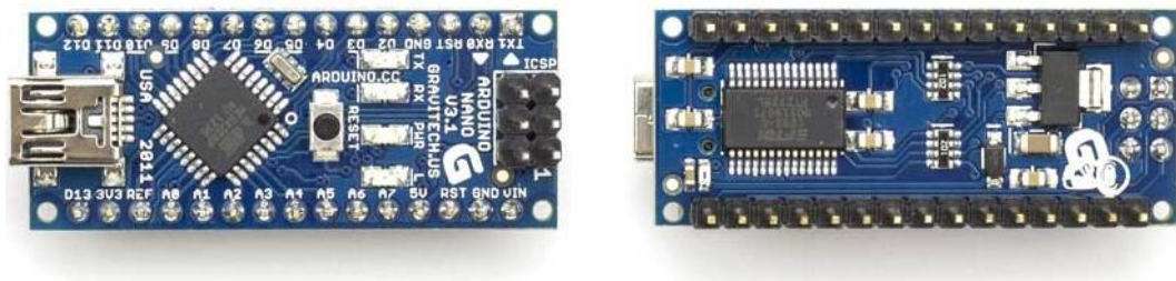
Figure 38. Arduino Nano board front (left) and rear [53].
