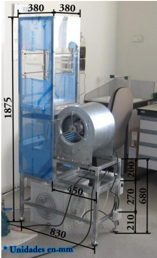
Figure 1. Illustration of the studied cooling tower installation.
