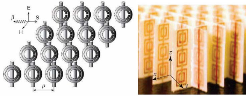
Figure 4.2: First experimental LH structures, constituted of TWs and SRRs. Reproduced from [Smith et al, 2000] and [Shelby et al, 2001]
