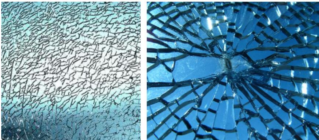
Figure 114 Typical example of fully-tempered (FT) glass breakage (Umberto GALLI, 2011)
