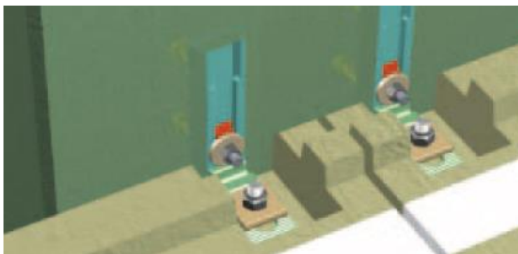
Figure 89 Horizontal panels suspended by pillars FO/00 (Ruredil. Construction chemicals and building technologies. “Fisis Earthquake-proof system for fixing panels”)
