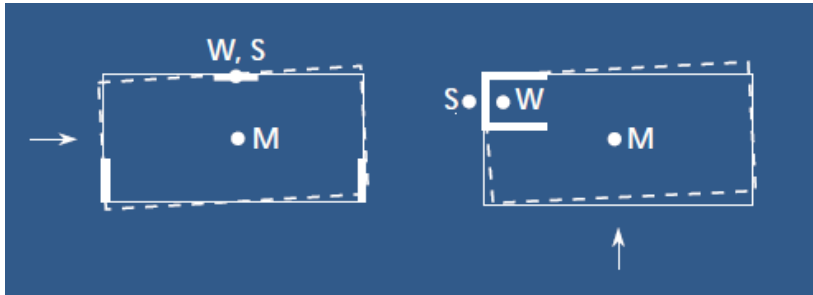
Figure 23 Asymmetric bracing (Hugo Bachmann, 2011)
