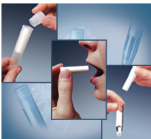
Figure 1. Saliva samples were collected using Salivette tubes. The students were instructed to chew the cotton wool Swab. Recovery of the saliva sample is achieved by returning the swab to the Salivette and centrifuging the container.
