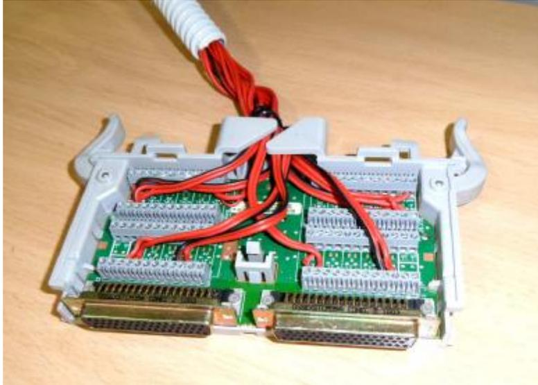
Fig. 62 Tarjeta multiplexora 34921A
