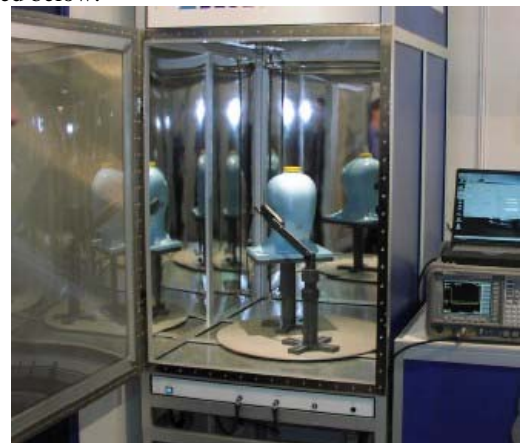
Fig. 7. RC800 Reverberation chamber at Carthagene.
