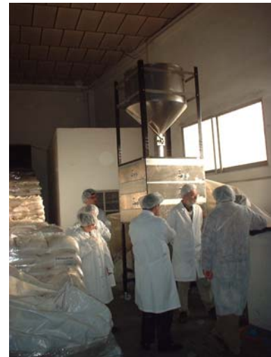
Fig. 2. The patent-protected rice disinfecting microwave unit at work.
