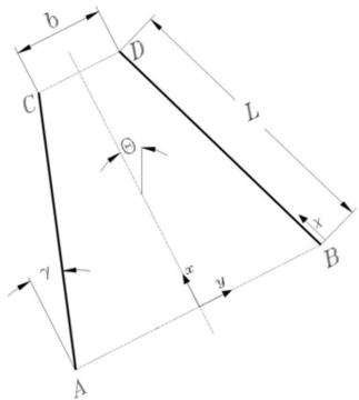
Fig. 1: Scheme of a converging sloped channel formed by walls AC and BD. The convergence angle is g, and the slope angle Q.
