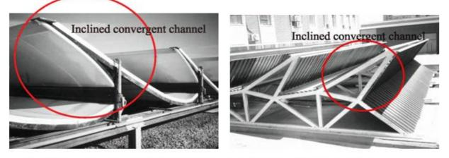
Fig. 2: Two experimental prototypes of the hydro-solar chimney that includes an inclined convergent channel.
