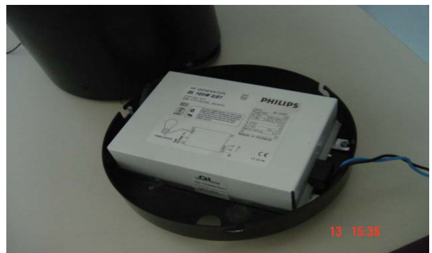
Figure 3. Rear side of the original luminaire with HF generator equipment
