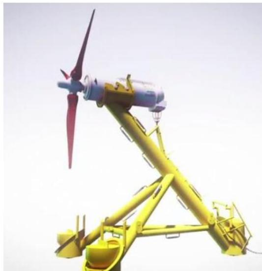
Figura 6.3: Turbina Andritz Hydro Hammerfest HS1000. Fuente: <https://conservatuplaneta.com>
