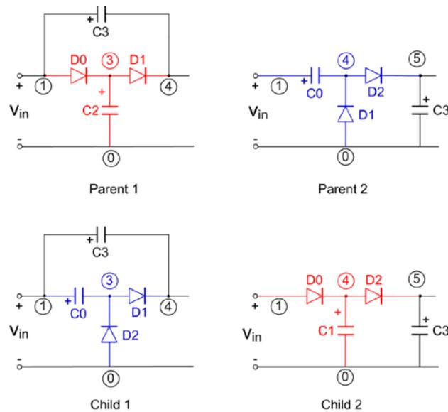
Fig. 3. Example of crossover between two parent circuits.
