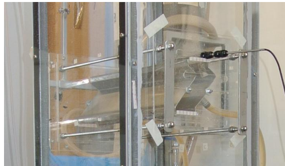
Figure 2. Image of the test section including the plates of the drift eliminator.
