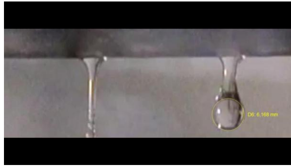
Figure 18. Image of experimental droplets leaving the separator plate. The experimental case is the V1Q1.
