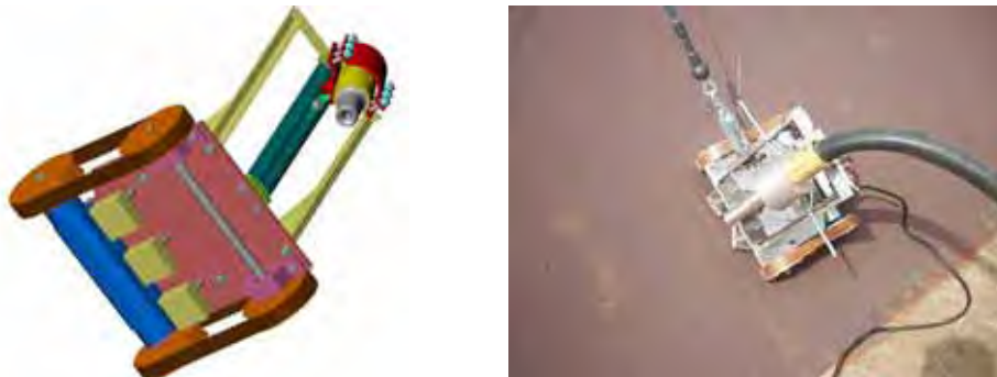
Figure 5. Lázaro I, CAD model and built prototype
