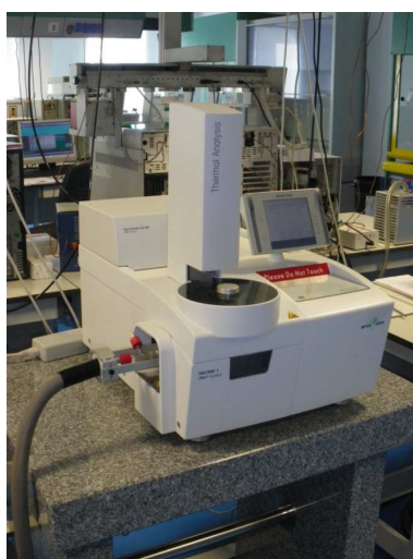
Figura 3.10: Termobalanza Mettler-Toledo TGA 1HT.
