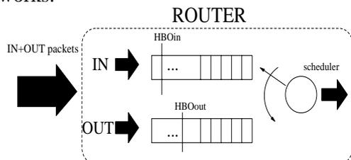
Fig. 1. Counters-Based Dual Queuing scheme.
