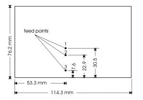
**Figure 4:** Probe-fed patch antenna on an infinite ground plane. Substrate: REXOLITE 2200, h = 1.59 mm,  $\varepsilon_r = 2.62$ ,  $tan\delta \approx 0.002$ .
