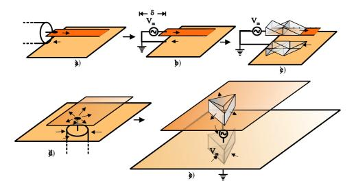
Figure 7: Attachment mode for patch antennas on fi nite ground planes. a) Colinear transition between a coaxial probe and a microstrip line. b) Delta-Gap voltage model applyed to a coaxial probe-fed microstrip line. c) Associated MoM description of the excitation model. d) Coaxial probe-fed patch antenna. e) Associated MoM description of the of the excitation of a probe-fed patch antenna.
