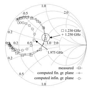
**Figure 9:** Measured versus simulated results for a perfectly balanced patch antenna:  $W_p = W_g = 120.1$  mm,  $L_p = L_g = 79.5$  mm,  $L_p = L_g = 80$  mm,  $X_p = 60$  mm,  $Y_p = 29$  mm. Substrate: RT/DUROID 5870, h = 1.57mm,  $\varepsilon_r = 2.33$ ,  $tan\delta = 0.0012$ . (increment 2.5 MHz clockwise)
