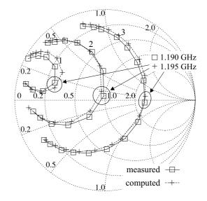
Figure 8: Measured versus simulated results for the patch antenna shown in Fig. 4, when the new excitation model is used:  $W_g = 214$  mm,  $L_g = 214$  mm. (increment 5 MHz clockwise, measurement reproduced from [James and Hall 1989])
