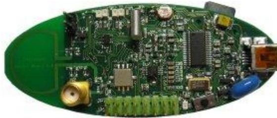
Figura 3.6: Nodo sensor EyesIFX
