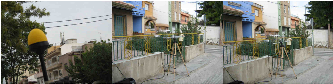
Figura 21. PM1: Banda Ancha (I) Pol Horizontal (C) Pol Vertical (D).
